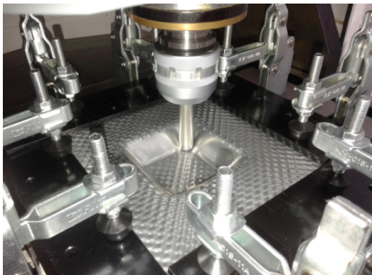
[Fig. 3] CNC-based incremental forming machine using cylindrical tool and toggle clamp jig
