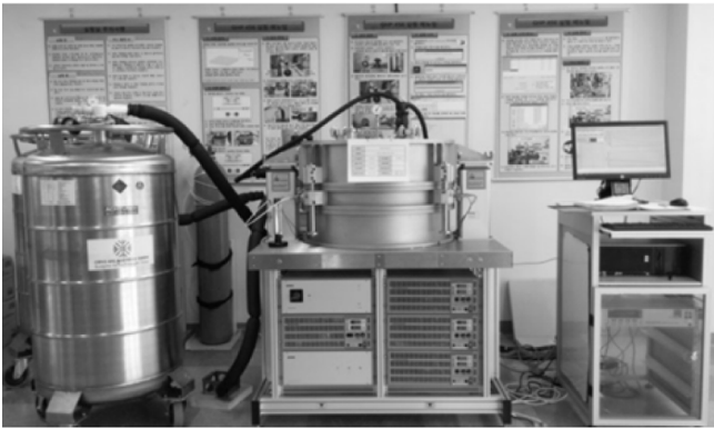
Fig. 3 Guarded hot plate method apparatus used in experiments
