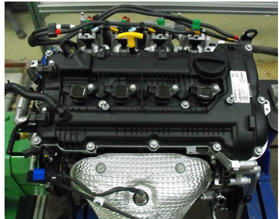
Fig. 1 Photograph of 2.0 LPLi nu Engine
