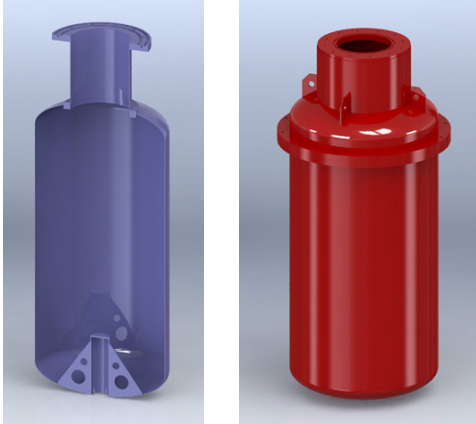
Fig. 3 Inner and outer tank of the hydrogen liquefier
