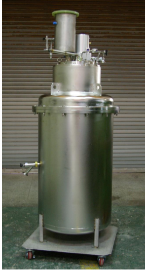
Fig. 6 Small scale hydrogen liquefier
