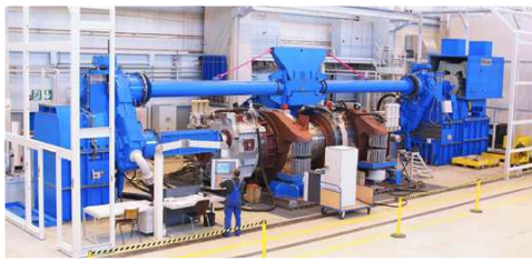
(b) Mechanical power-circulation test rig
