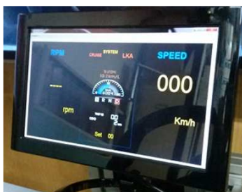
Fig. 6 A 10 inch LCD monitor to simulate a car instrument cluster
