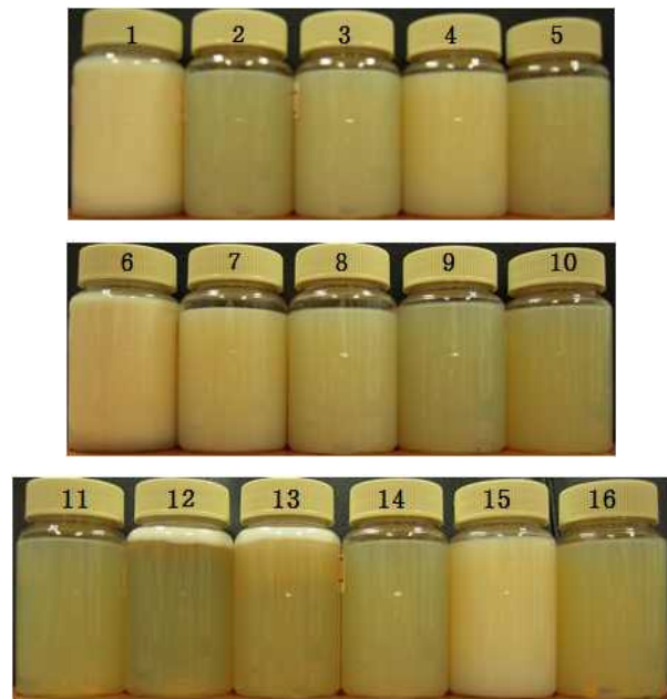
[Fig. 1] Photograph of emulsions prepared Tween 80/Span 80/candelilla wax/oil/water, 1: Waglinol 812, 2: KAK 99, 3: NS-CIO, 4: ODM, 5: ICEH, 6: Eutanol G, 7: TOG, 8: ICM-R, 9: LP 70, 10: Pripure 3759, 11: Isopar H, 12: Silicone 200/100cs, 13: Silicone 200/6cs, 14: DC 345, 15: Jojoba oil, 16: Silicone 556.
