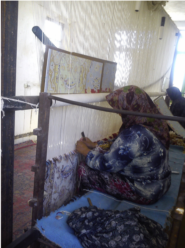
Fig. 2. A woman sitting on a wooden flat; there is not adequate space in front of her legs for free leg movements.
