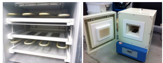
(b) Plasma treatment and Thermal release process
