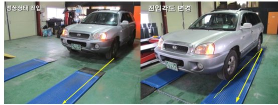
Fig. 5 Testing on dynamic braking force inspection system
