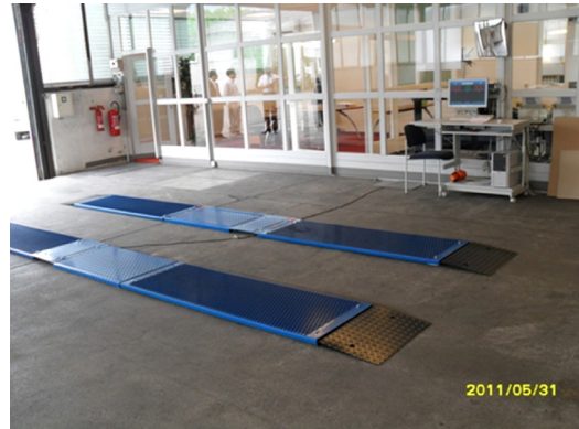
Fig. 4 Dynamic braking inspection system
