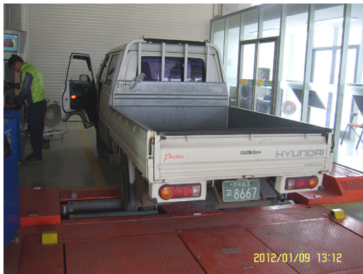
Fig. 3 Static braking force inspection system
