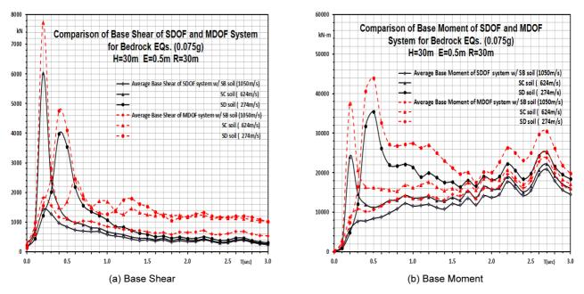
Fig. 7. Comparison of Base Shear and Base Moment of SDOF and MDOF systems
