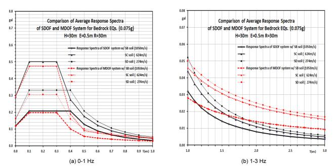
Fig. 5. Comparison of Response Spectra of SDOF and MDOF systems
