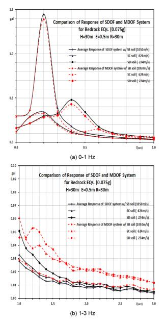
Fig. 3. Comparison of Responses of SDOF and MDOF Systems
