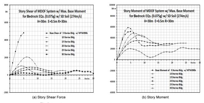
Fig. 9. Story Shear Force and Moment of MDOF system with Max. Base Moment
