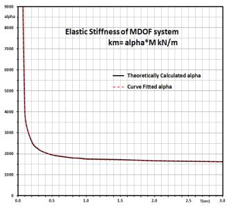
Fig. 4. Elastic Stiffness for a MDOF System.
