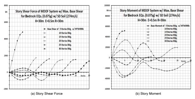
Fig. 8. Story Shear Force and Moment of MDOF system with Max. Base Shear Force
