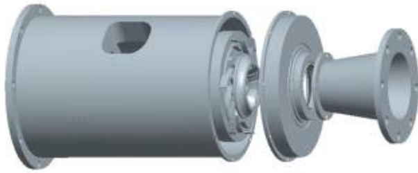
Fig. 1 Schematic view of inline francis turbine model
