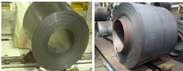
(a) Good coiling shape. (b) Bad coiling shape.
