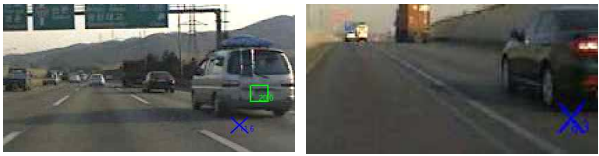
(a) Performance difference of position measurement. (b) Misdetection of vehicle out of vision sensor's field of view.
