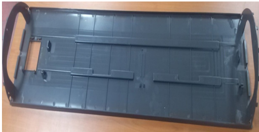
Fig. 7 Result of injection molding without undercut processing unit from rib
