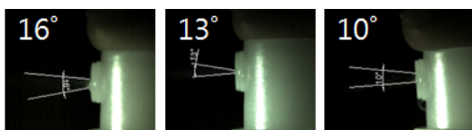
Fig. 7 Injection angle according to orifice length
