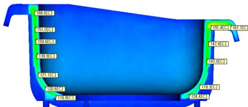
Fig. 11 Different temperature in inside of molding
