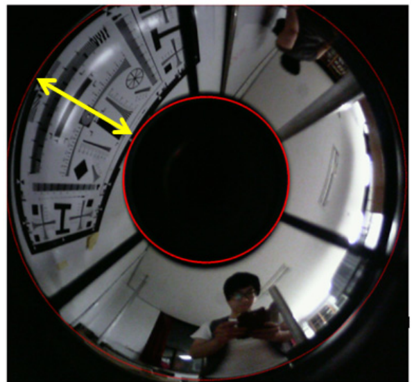
FIG. 12. The measurement of field of view of the catadioptric omnidirectional optical system by the image of ISO 12233 chart.
