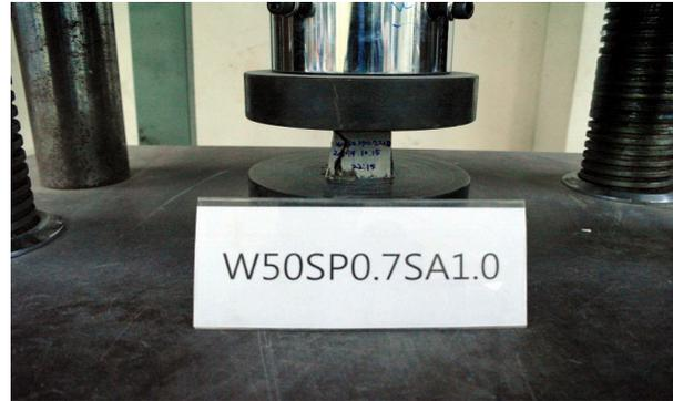
Fig. 6 Test for Compressive Strength of Mortar
