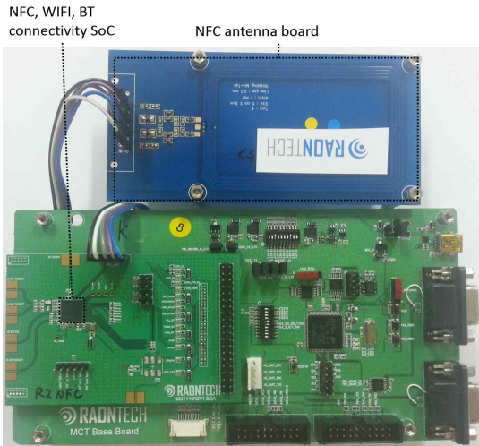
Fig. 8. Test board for verifying the NFC modem.
