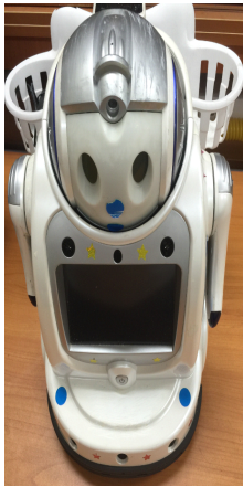
Fig 1. 2DOF two-wheeled balancing mobile robot.
