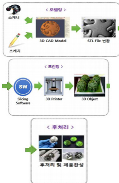
(Fig. 1) 3-Step Process of 3D Printing[10]
