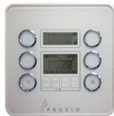
Fig. 6. Standby power shut-off switch.
