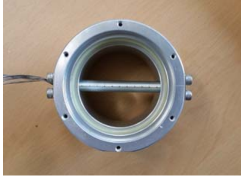
Fig. 3 Schematic of thermocouple rack with airfoil structure (11 thermocouples)
