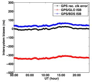
Fig. 5. The temporal variations of GPS/GLONASS ISB and GPS/BeiDou ISB.
