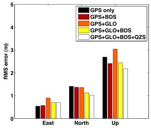
Fig. 4. Position RMS errors calculated by multi-GNSS combinations.
