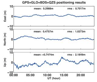
Fig. 2. Combined GPS+GLO+BDS+QZS standard point positioning error.
