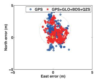
Fig. 3. Comparison of the horizontal position errors between GPS and GPS+GLO+BDS+QZS.
