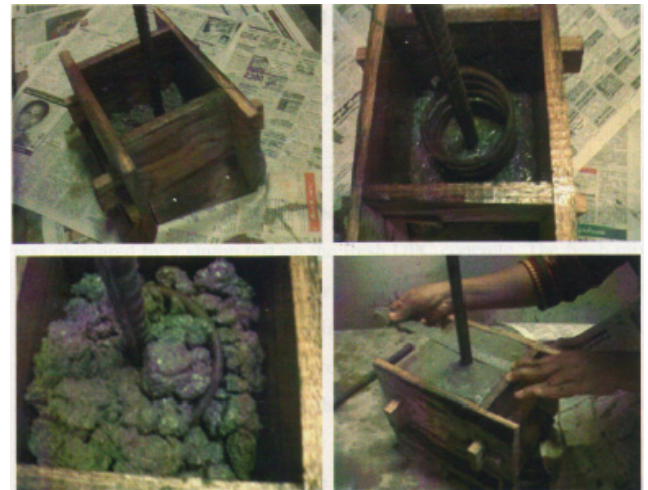
Fig. 2 Specimens for pull-out test
