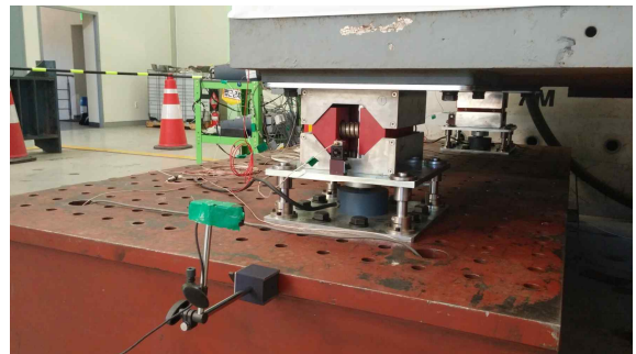
(b) Isolator and test zig
