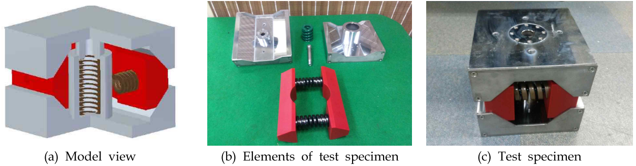
Fig. 1. Friction wedge type vibration isolator
