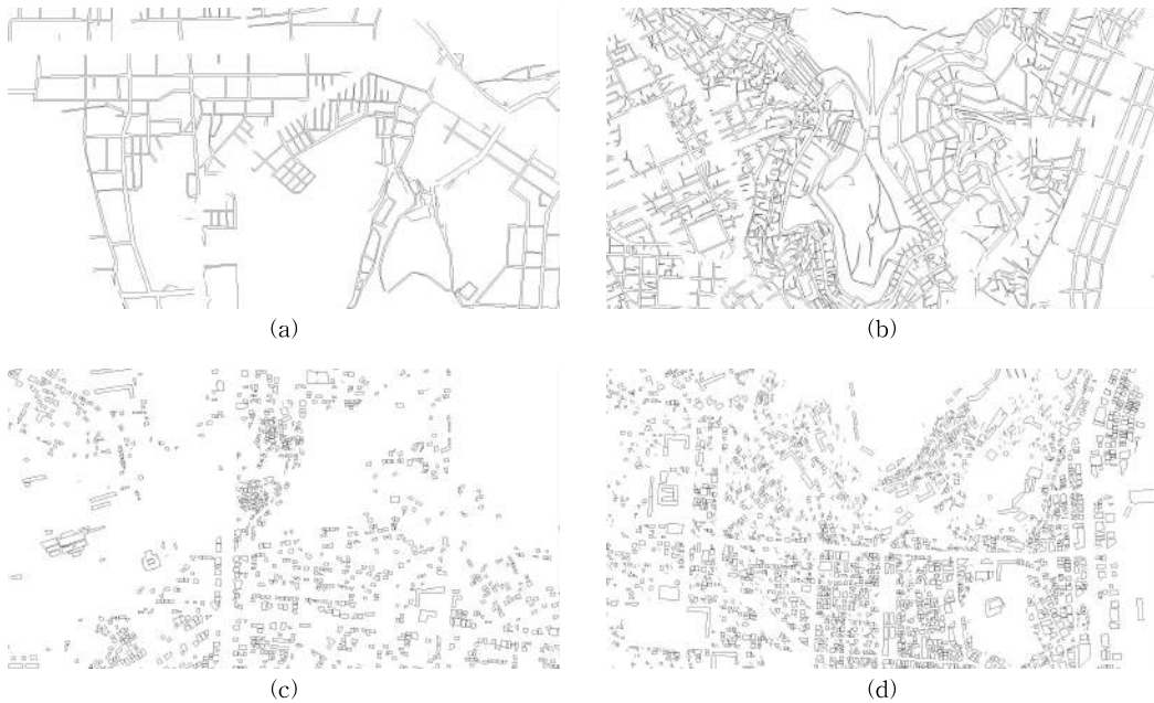
Fig. 6. Shape changes with \epsilon=5 using DP algorithm: (a) Polyline layer for Changwon (b) Polyline layer for Daegu, (c) \epsilon=9 , (c) Polygon layer for Changwon, (d) Polygon layer for Daegu.
