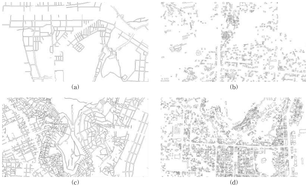
Fig. 7. Compressed map by vector data compression based on bin classification; (a) Polyline layer, (b) Polygon layer for Changwon and (c) Polyline layer, (d) Polygon layer for Daegu.
