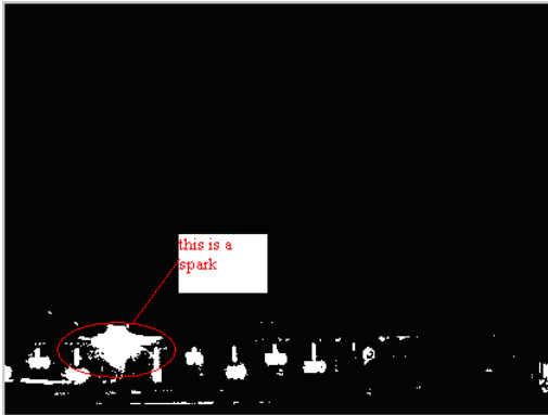
Fig. 6. Example of the spark image after binarization.
