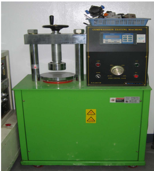
Fig. 2. Compressive strength testing machine.
