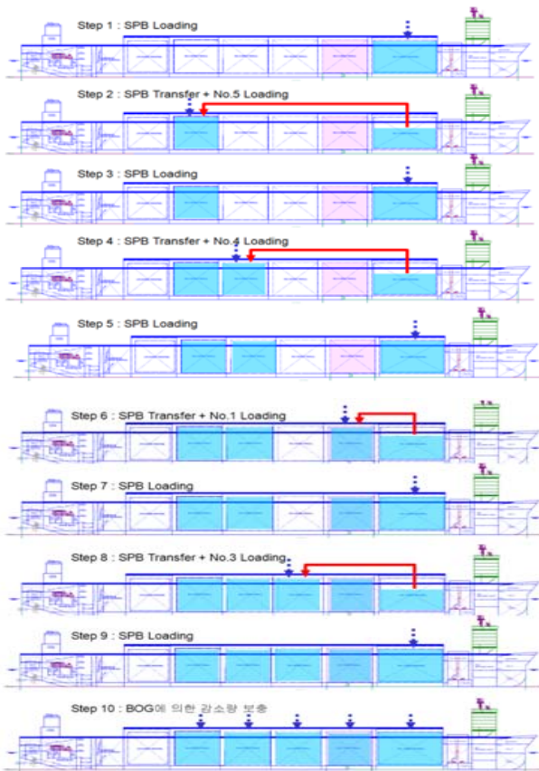
Figure 5: LNG operation procedure
