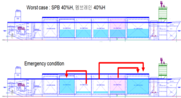
Figure 7: Emergency LNG transfer (Combined containment system)
