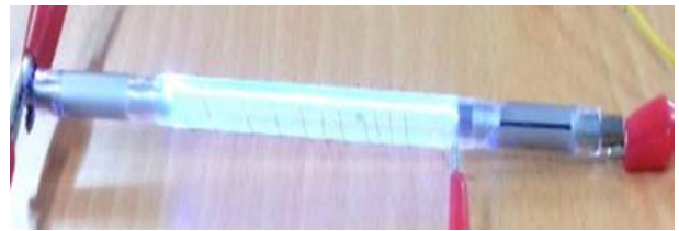
Figure 4: Simmer triggering of xenon flashlamp
