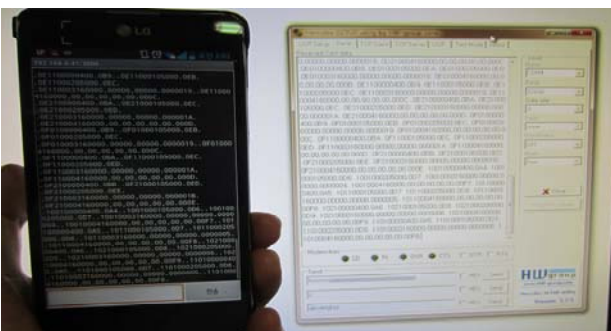
Figure 14: NMEA2000/WIFI data transfer test
