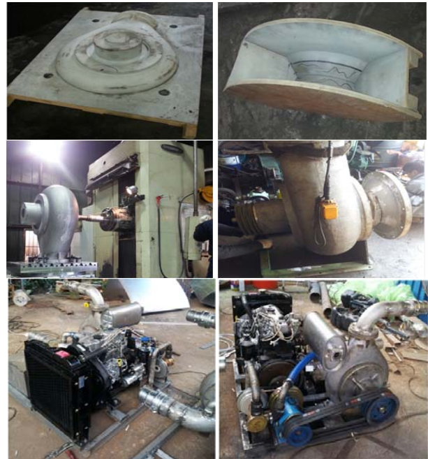
Figure 19: Prototype production of drainage pump system
