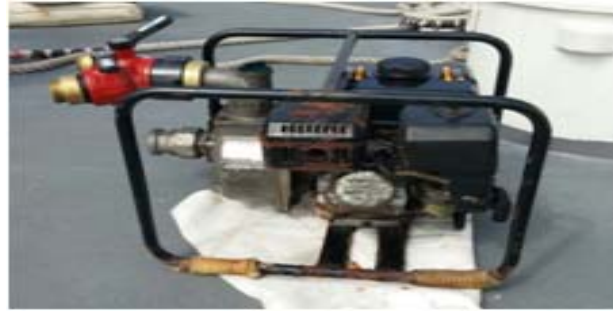
Figure 2: Existing drainage pump of Korea coast guard
