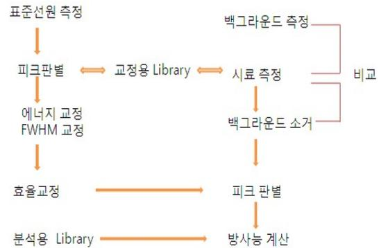
**Fig. 3.** Procedure of the gamma-ray spectrometry analysis.
