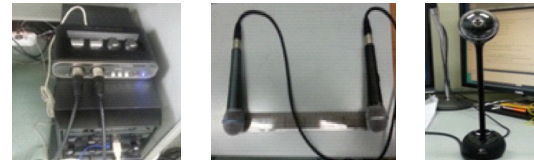
(a) Multichannel audio interface (b) Two cardioid microphones (c) Pan-tilt camera
