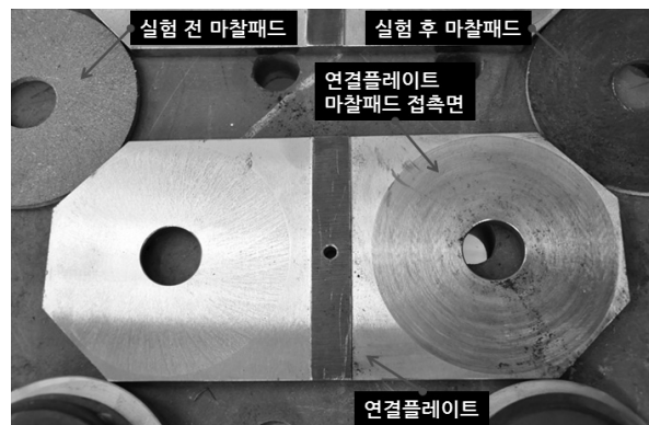
Fig. 5 Connection plate and Friction Pad before and after test
