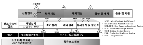
[Figure 1] ROK defense acquisition system and naval ship design process
