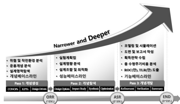
[Figure 2] A roadmap of early-phase ROKN ship design process
