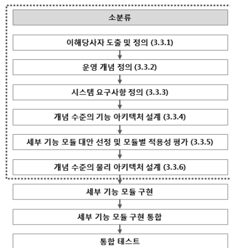
[Figure 1] SE based design process for pilot platform
