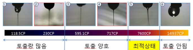
Fig. 4 Electrospinning with respect to viscosity
