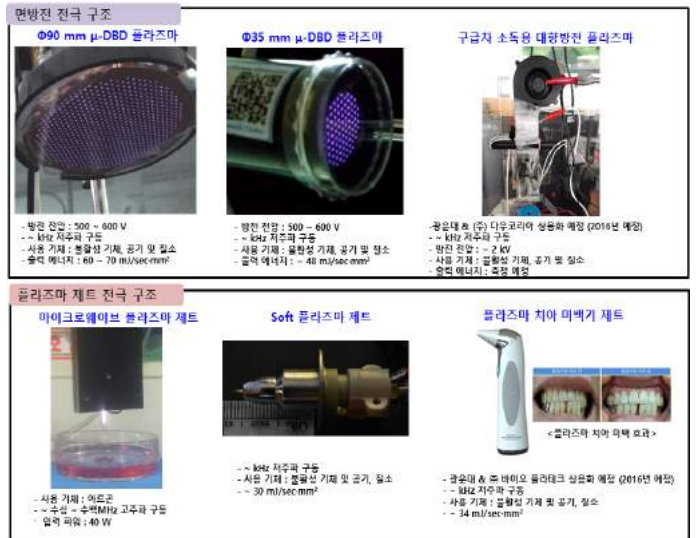
[Fig. 4] Nonthermal atmospheric pressure plasma sources for plasma bioscience and medicines
