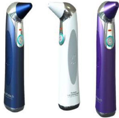
[Fig. 11] Portable non-thermal atmospheric pressure plasma jet for tooth bleaching
