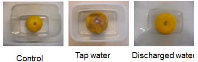
[Fig. 8] Sterilization by plasma discharged water. The mandarins in 2 weeks at 30°C after washing.
