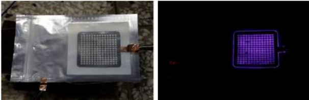
[Fig. 7] Plasma generation inside sealed packages by coating thin film electrode on inner surface of packaging material
