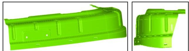
Fig. 1 3D model of seat side cushion panel
