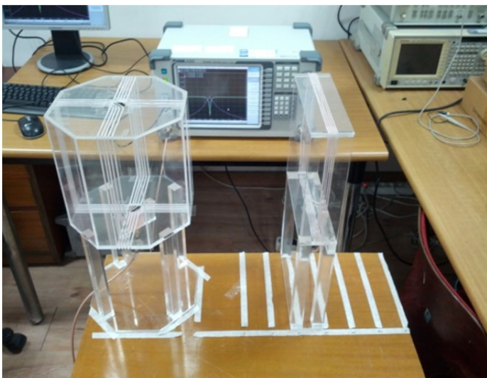
Fig. 5. Transmitter and receiver at 200 mm at 0^\circ .
