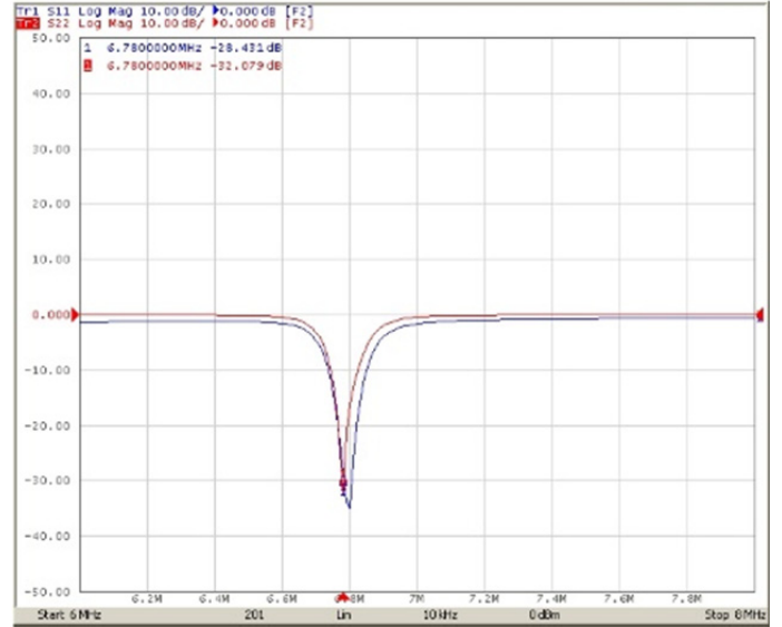
Fig. 6. Measured reflection coefficient at 200 mm at 0^\circ .
