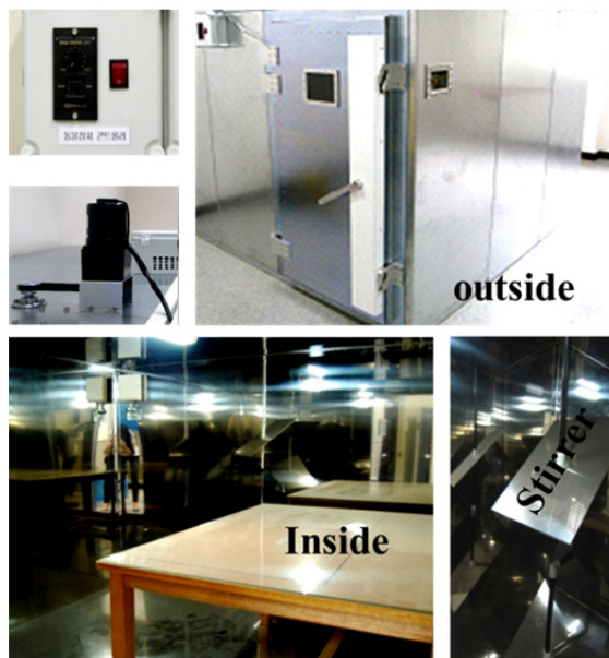
Fig. 1. A whole-body 915-MHz radiofrequency identification (RFID) exposure system. This system was designed for small animal experiments with a continuous wave 915-MHz RFID signal generation using a reverberation chamber.
