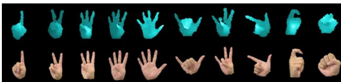
Fig. 5. Hand posture database used in this study, which captured by Kinect sensor (the first row are the depth images and the second row are the corresponding color images)
