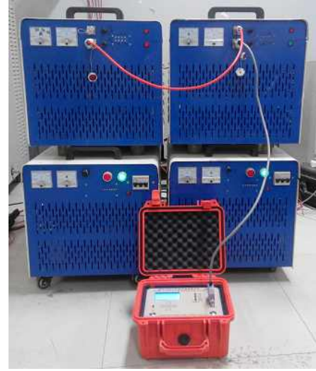
Fig. 12. Photo of a 40 kW transmitter.
