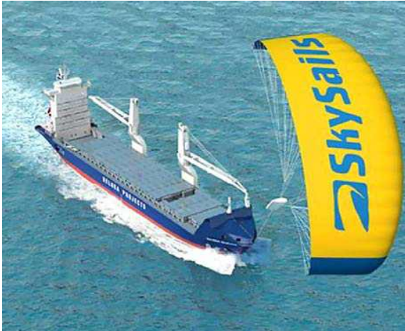
Fig. 1. The Skysails system with a parafoil ( http://www.skysails.info )
