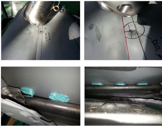
Fig. 7. Impact beam after collision experiment test.
