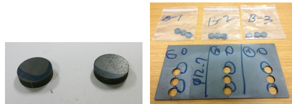
Fig. 6 Specimens and diffusion-bonded plate for LFA.
